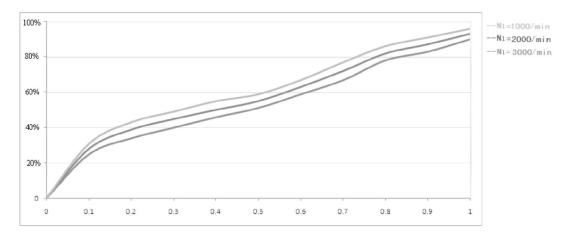
Hysteresis curve: Delay detection is to reverse the reducer stiffness. Get the hysteresis curve by testing. When detecting, the reducer input end is fixed, and then in the two rotation direction output were continuously loaded into the T<sub>2B</sub> maximum acceleration torque, and then gradually unloading, instrument record the moment imitation difference angle, the curve is a closed curve, from which we can calculate the backlash reducer (it) and torsional stiffness (C<sub>21</sub>).
